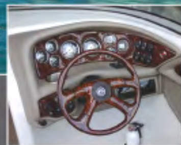
Upgraded vinyl wrapped dash and gauge cluster with stainless steel bezels and woodgrain dash with Executive solid wood steering wheel.
