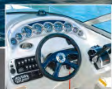
Fully instrumented helm features deluxe reduced glare gauges with stainless steel bezels.
