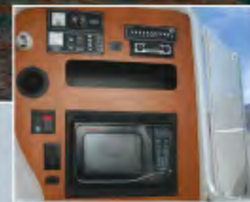
Forward cabin bulkhead houses the stereo controls, shore power panel, circuit breakers, AC controls, 120 V receptacle and microwave.
